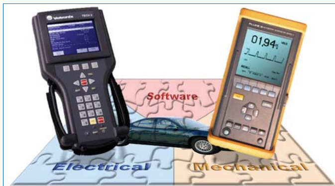
The Dynamic Duo: The scantool offers a dynamic perspective of the system's software view. The lab scope offers a dynamic perspective from the circuit's view.
