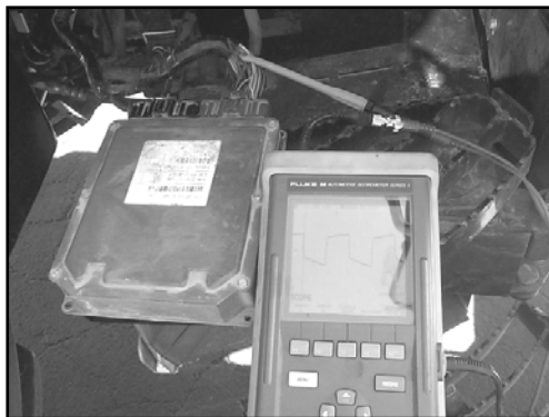
Checking the engine speed output signals from the ACU
