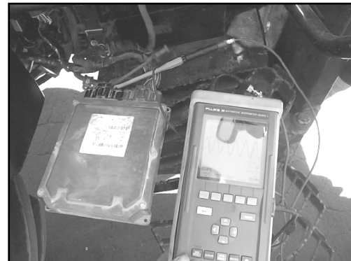
Testing the engine speed sensor signal at the ACU
