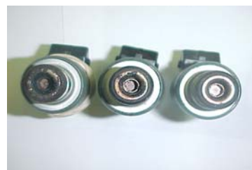
Carbon build-up reduces flow
