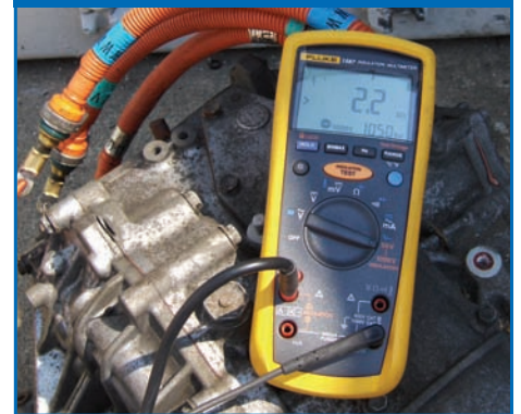
Figure 5: Second transaxle with good MG windings
