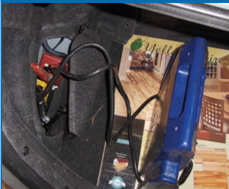
Figure 2: Installing battery pack on AGM battery
