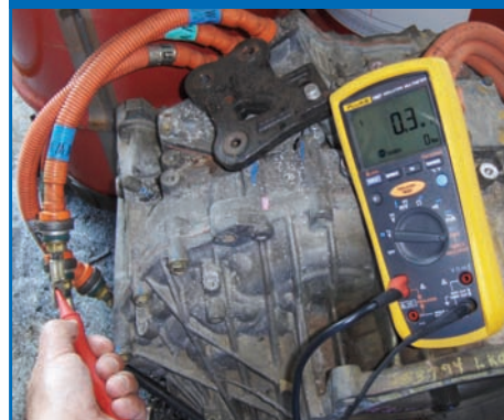
Figure 4: Hybrid transaxle with shorted MG windings
