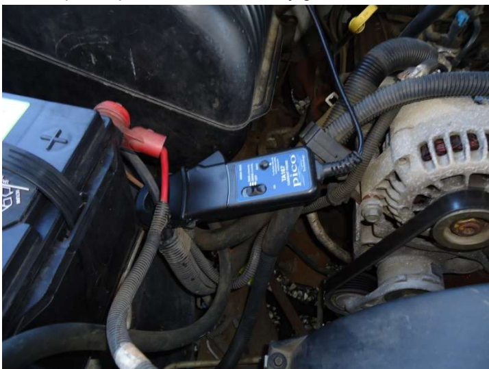
Amp clamp connected to battery ground cable.
