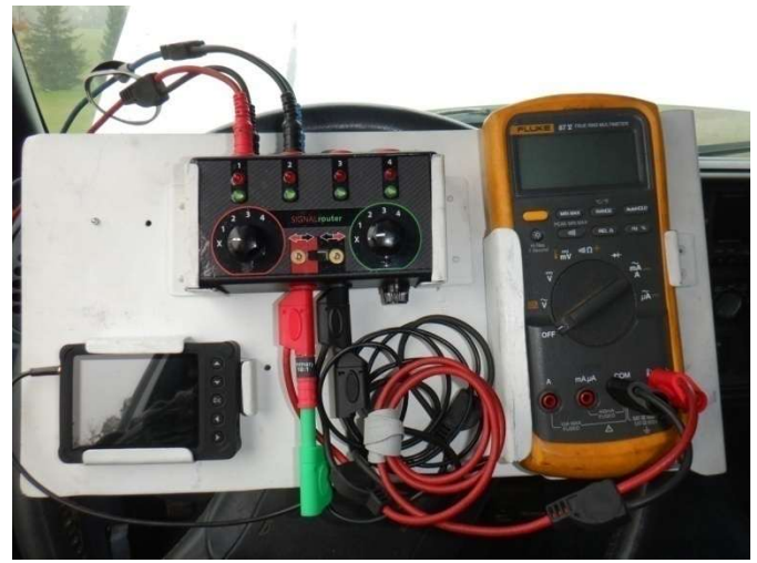
Photo 3 : Add a 10:1 Attenuator to capture a fuel injector pattern or any other relay or solenoid pattern.
