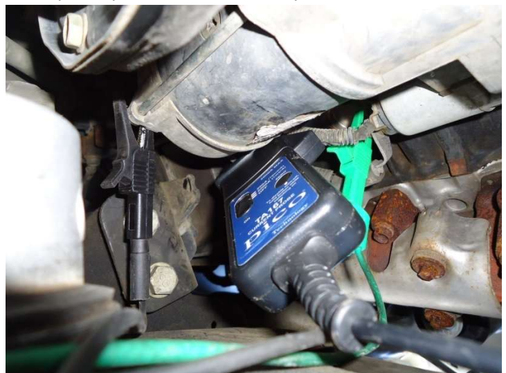
Amp clamp connected to starter power cable.
