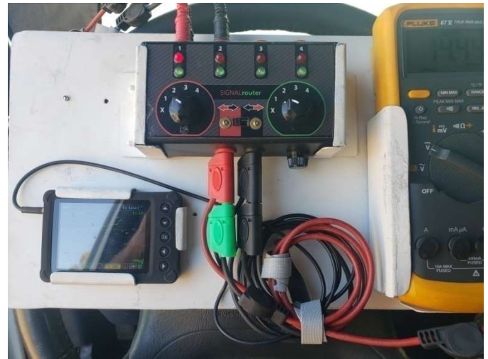
Photo 1 : Connections set up for the Cranking Voltage Test See page ## for pattern examples.
